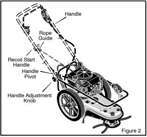
5. To attach the **recoil start handle** to the **rope guide**, twist the rope through the **rope guide** mounted on the right side of the handlebar.
